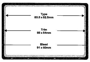
Measurements are in mm
