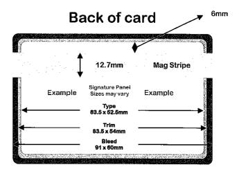
Measurements are in mm
